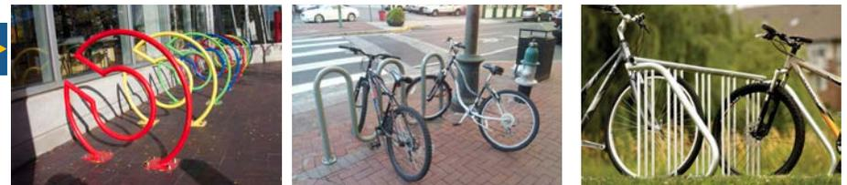
*Use racks with two points of contact, such as the Columbus “C” rack, left. Do not use racks such as “wave” racks, middle, or “wheel-bender” racks, right.*
