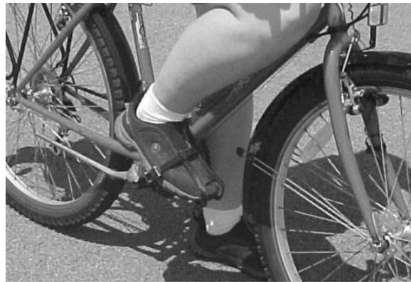
The right pedal is at the 2 o'clock position. The left pedal can also be used to push off, depending on the rider's preference.
